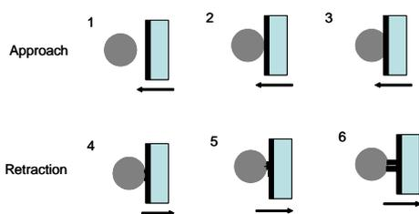
Stored energy or area A can be used as an estimate for the grease cohesion or plastic resistance against indentation.
