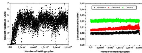
Greases A, B and C prevent this increase. Further distinction is visible in the wear tracks : grease C is more effective in reducing the total wear than grease A.
