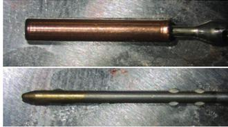
This may cause fretting damage and this damage in turn may create wear particles that isolate the electrical contact, or damage an electrically conductive coating, like gold.
